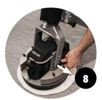
Pull latch to loosen body.
